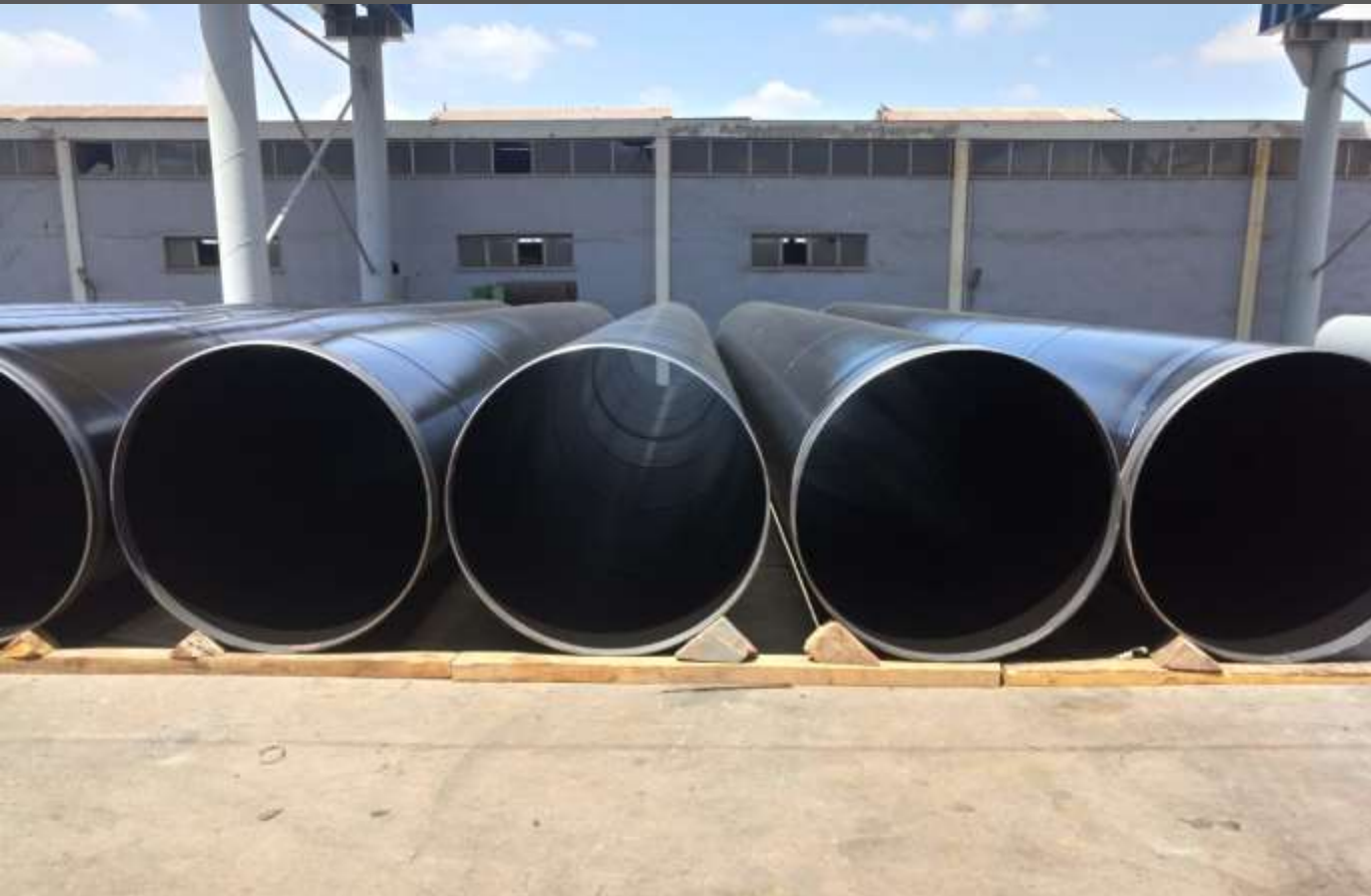
SPIRAL STEEL WATER PIPES TO LEMNOS ISLAND / GREECE
