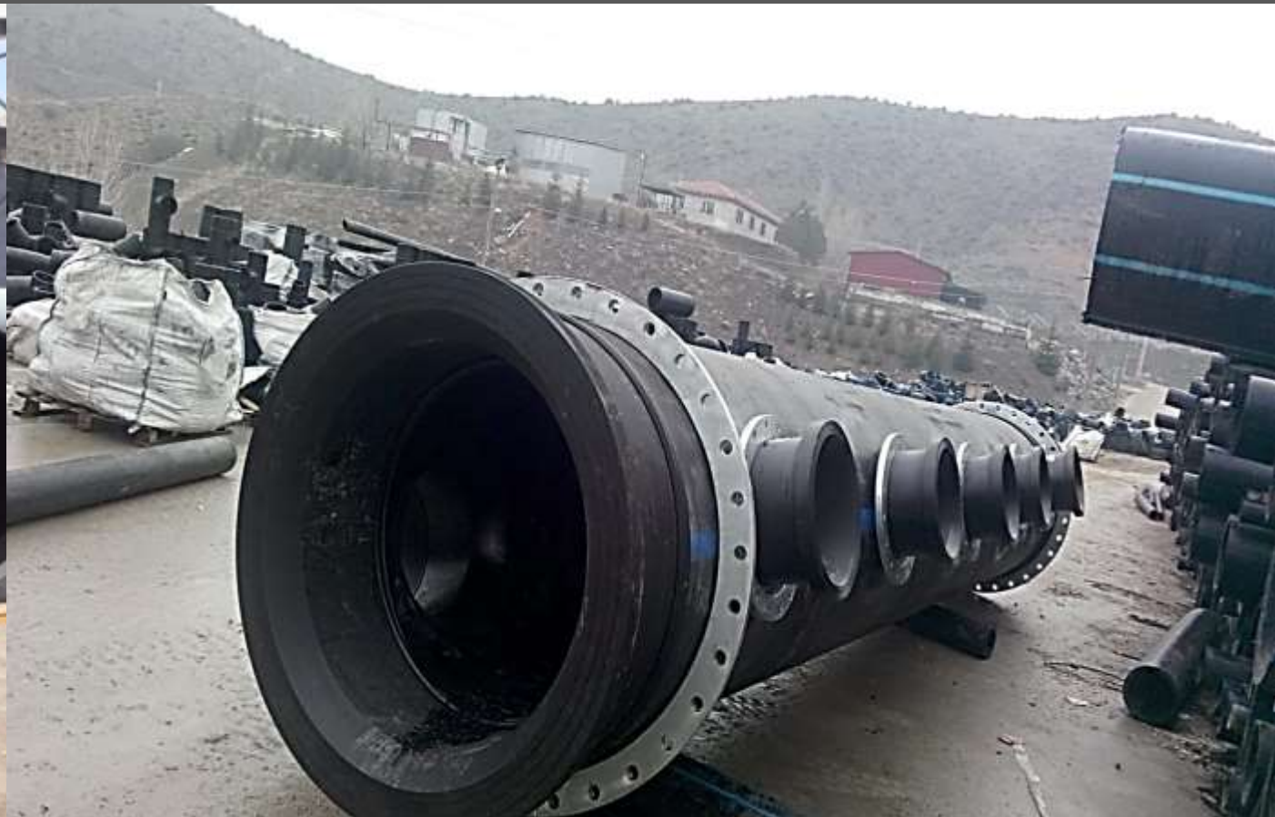
HDPE SEA-WATER COLLECTOR PIPES KOS ISLAND / GREECE
