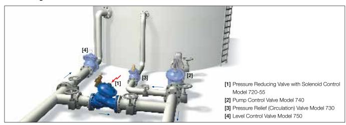
The Model 720-55 is installed as a by-pass between the reservoir supply line and the pump discharge line to the distribution network providing four major advantages:
